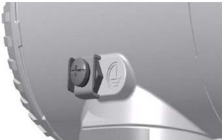
Figure 19 Ground connection on transmitter housing
