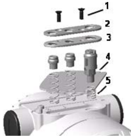
Figure 15 External push button assembly components
